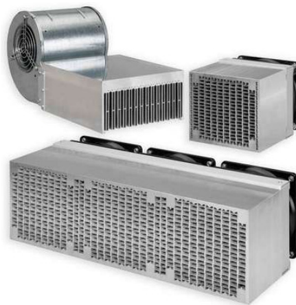
Illustration 4: Compact heat exchanging surfaces result in an extremely effective honeycomb structure which often provides very good heat distribution within the unit.
